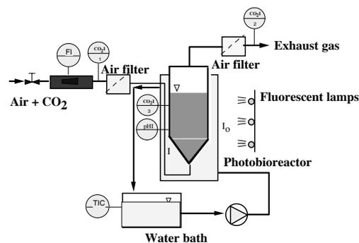
Figure 1. Experimental apparatus
