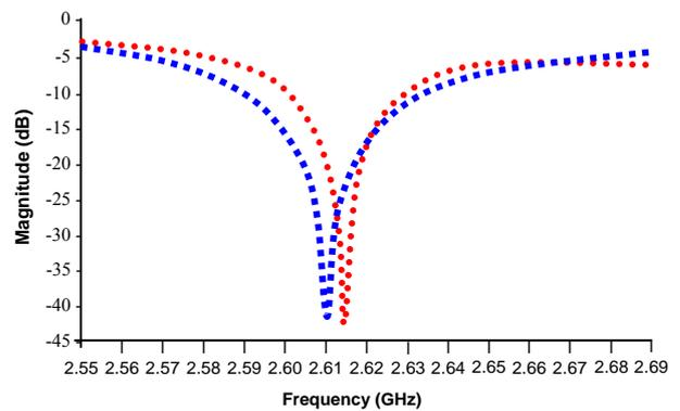
Figure 5. Impedance Bandwidth of Antenna between Measured (●), Simulated (■)
