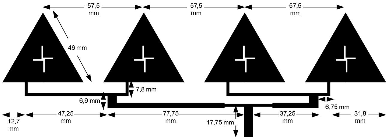
Figure 4. Final Antenna Design
