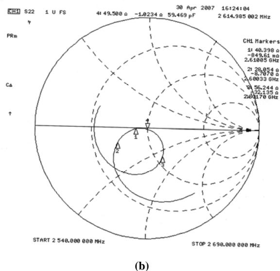
Figure 6. Input Impedance (a) Simulation Result, (b) Measurement Result
