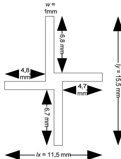
Figure 2. Shape and Dimensions of the Cross Slot
