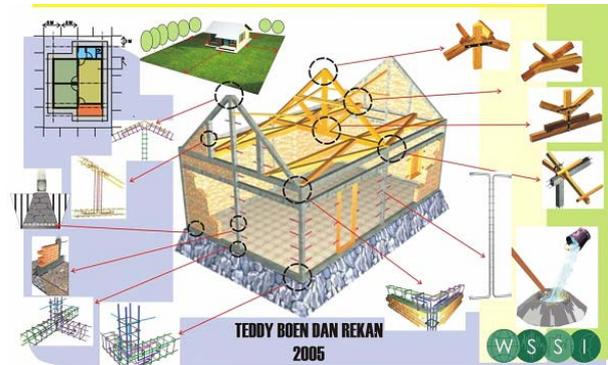
Figure 2. Building the Earthquake Safe Masonry House [7]
