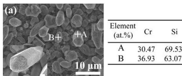
Fig. 3. SEM Images and Corresponding EDS Results of the  $\text{CrSi}_2$  Sample Grown at 750 °C with 0.05 g of  $\text{CrCl}_2$ . Magnified SEM Image of a Microrod in (a) Shown in the Inset
