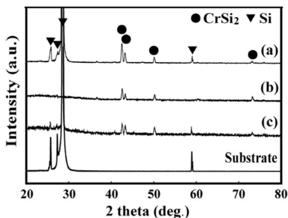
Fig. 2. XRD Spectra of the  $\text{CrSi}_2$  Samples Grown at (a) 750 °C with 0.05 g of  $\text{CrCl}_2$ , (b) at 750 °C with 0.1 g of  $\text{CrCl}_2$  and (c) at 700 °C with 0.1 g of  $\text{CrCl}_2$
