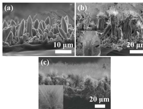
Fig. 1. Cross-sectional SEM Images of the  $\text{CrSi}_2$  Samples Grown at (a) 750 °C with 0.05 g of  $\text{CrCl}_2$ , (b) at 750 °C with 0.1 g of  $\text{CrCl}_2$  and (c) at 700 °C with 0.1 g of  $\text{CrCl}_2$ . Magnified SEM Images of the Nanowires in (b) and (c) Shown in the Inset
