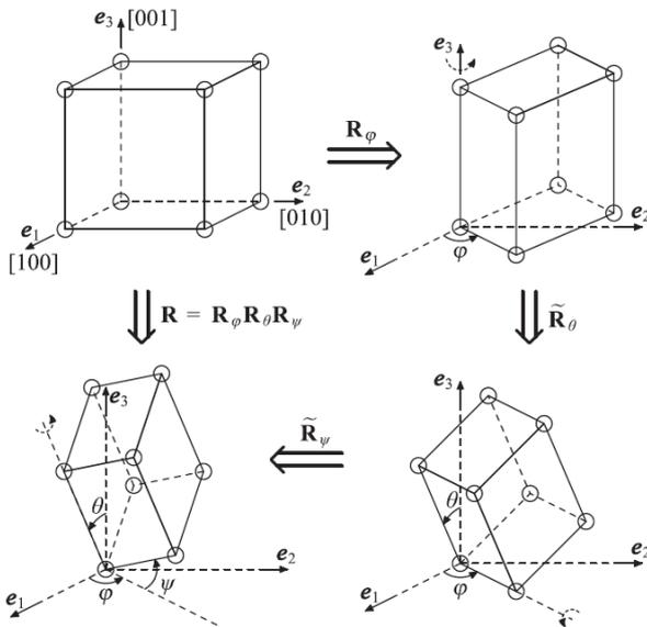
**Figure 2. Schematic Illustration of the Rigid Rotation Motion Operation in Euler Angles to Define the Crystallographic Orientation**
