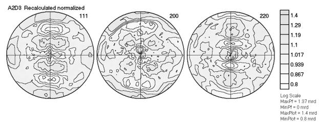
**Figure 5. Normalized Pole Figures (111), (200), and (220) for the A2D3 Sample**
