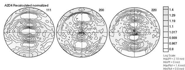
**Figure 5. Normalized Pole Figures (111), (200), and (220) for the A2D4 Sample**
