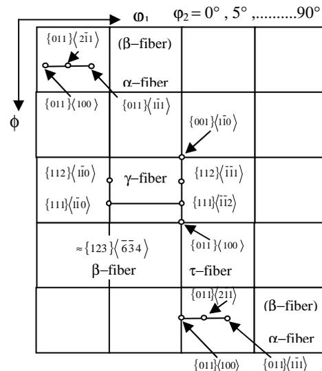
Figure 1. Some Relevant Orientation and Texture Fiber that Occur in Strip Cast & Hot-rolled Stainless Steels [2]
