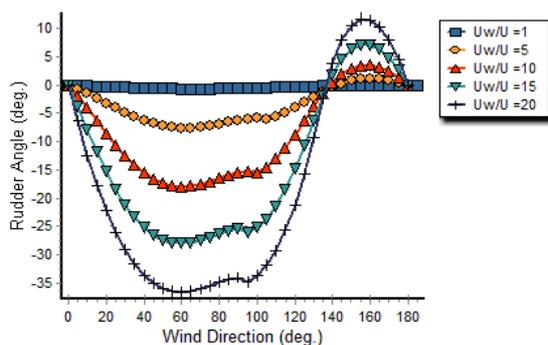
Figure 6. Rudder Angles in a Steady State Condition
