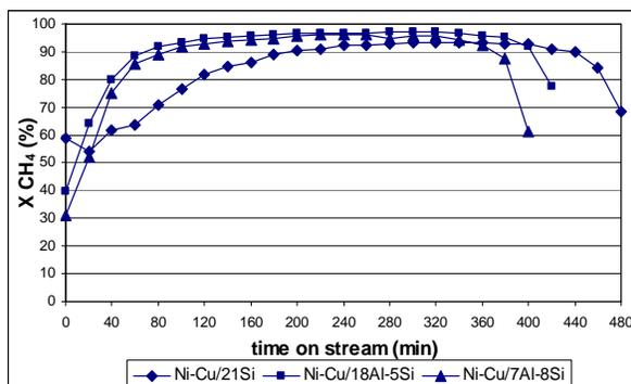
Figure 2. Methane conversion vs. time on stream
