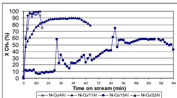
Figure 1. Methane conversion of Ni-Cu/Al catalysts
