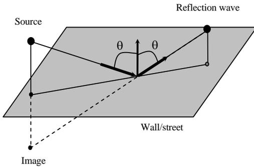
Figure 8. Reflection mechanism
