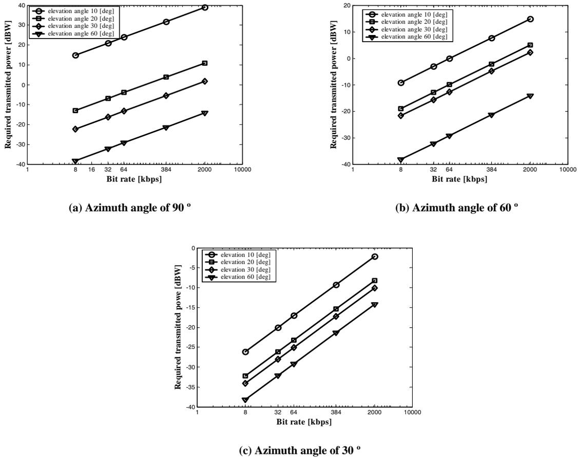
Figure 12. Required transmitted power at the SPF
