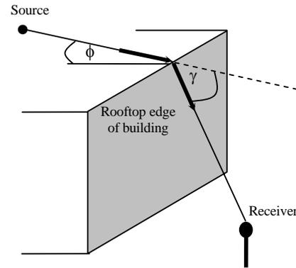
Figure 9. Diffraction mechanism
