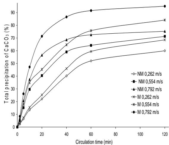
Figure 4. The Influence of Flow Rate Toward the Total Precipitation of  $\text{CaCO}_3$  (B : 5.2 kg,  $L_m$  0.35 m,  $\text{Ca}_i$  : 0.004 M, Initial pH of Solution 64, V : 240 mL and T : 28°C).
