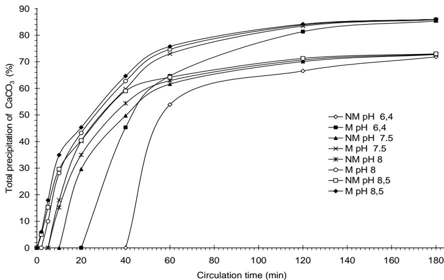
**Figure 2.** The Influence of the pH of the Solution toward the Total Precipitation of CaCO<sub>3</sub> on Non-Magnetized Sample (NM) and Magnetized Sample (M) (Magnetic Strength: 5.2 kg, Magnet Length (L<sub>m</sub>): 0.35 m, Flowrate (v): 0.554 m/s, Initial Concentration CaCO<sub>3</sub> (Ca<sub>i</sub>): 0.004 M, Sample Volume (V) 240 mL, and Temperature: 28°C).
