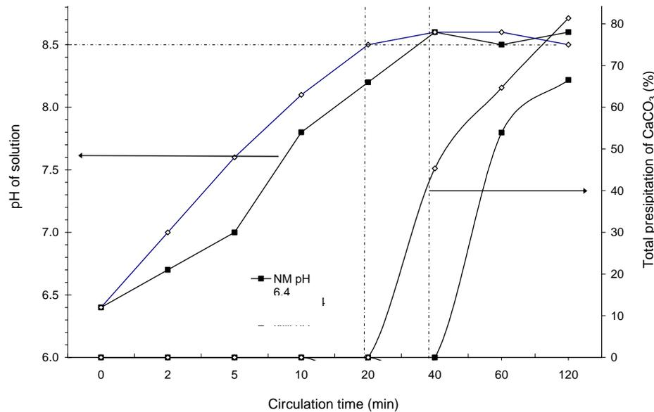
Figure 3. The Total Precipitation of  $\text{CaCO}_3$  the pH of Solution (B : 5.2 kg,  $L_m$  0.35 m, v : 0.554 m/s,  $\text{Ca}_i$  : 0.004 M, Initial pH of Solution: 6.4, V : 240 mL, and T : 28°C).
