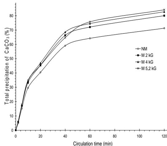
**Figure 5. The Affect of the Magnetic Field Strength Toward the Total Precipitation of CaCO<sub>3</sub> (L<sub>m</sub>: 0.35 m, v: 0.554 m/s, Ca<sub>i</sub>: 0.004 M, Initial pH of Solution: 6.4, V: 240 mL, and T: 28°C).**
