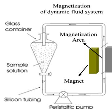
Figure 1. Schematic of the Experimental Treatments System
