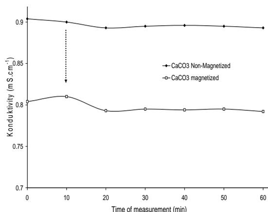
**Figure 7. The Affect of Magnetic Field on Solution Conductivity of CaCO<sub>3</sub> after 10 Minutes of Circulation (B: 5.2 kg, L<sub>m</sub>: 0.35 m, v: 0.554)**
