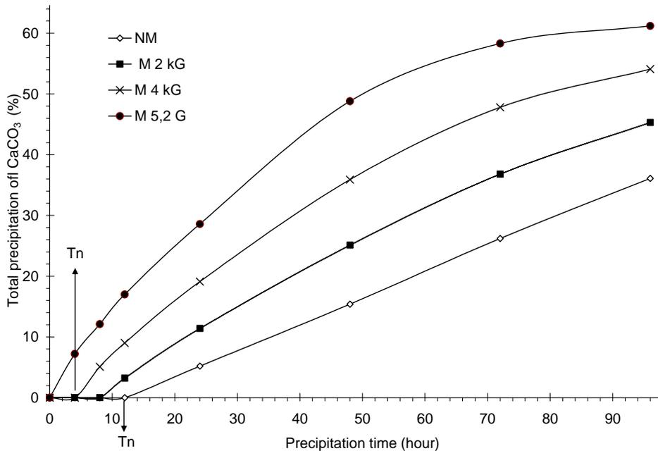
**Figure 6. The Affect of Magnetic Field Strength Toward the Toward the Total Precipitation of CaCO<sub>3</sub> (t<sub>s</sub>: 10 Minutes, L<sub>m</sub>: 0.35 m, v: 0.554 m/s, Ca<sub>i</sub>: 0.004 M, Initial pH of Solution: 6.4, V: 240 mL and T: 28°C).**
