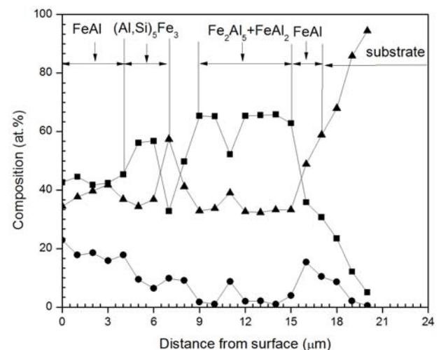
Figure 6. EDS Line Scan Analysis on the Cross-section of Aluminide Layer for the Aluminized Steel Oxidized for 9 h, Al (■), Si (●), Fe (▲)
