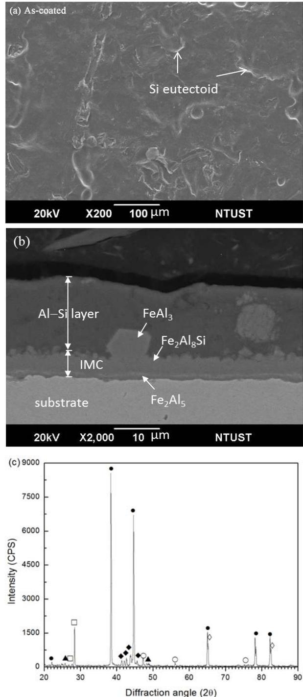
Figure 4. (a) SEM of Surface Morphology, (b) BEI of Cross-sectional Micrograph and (c) XRD Patterns as Coated Specimen, FeAl<sub>3</sub> (□), Fe<sub>2</sub>Al<sub>8</sub>Si (◆), Fe<sub>2</sub>Al<sub>5</sub> (○), Al (●), Si (▲), α-Fe (◇)
