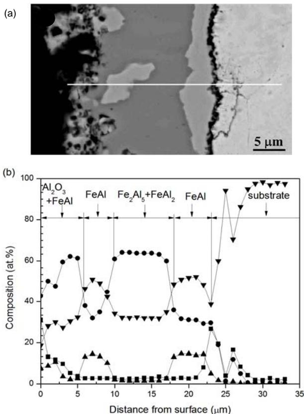
**Figure 7. (a) BEI of Cross Sectional Micrograph of the Aluminized Steel and (b) Corresponding to EDS Results of Elemental Composition of O (■), Al (●), Si (▲), and Fe (▼) for the Aluminized Steel After 49 h Exposure**
