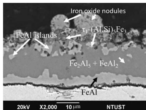
Figure 2. BEI of Cross-Sectional Micrograph Showing the Iron Oxide Nodules Growth on the Aluminized Steel Exposed to Ethanol Combustion Product at 700 °C for 9 h
